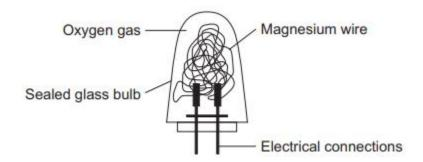
When a photograph is taken, an electric current flows through the magnesium. The magnesium burns very brightly and very quickly. A white powder called magnesium oxide (MgO) is formed. A student wanted to find out if the mass of the flash bulb changed when it was used.
