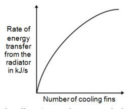
The number of cooling fins affects the rate of energy transfer from the radiator.
