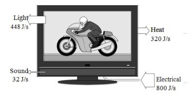
(a) (i) Use the information in the diagram and the equation in the box to calculate the efficiency of the TV.
