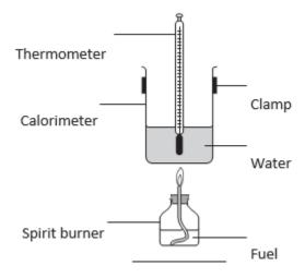
The heat produced when each fuel was burned was used to raise the temperature of 100 g of water. The student noted the mass of fuel burned, the increase in temperature and whether the flame was smoky.
