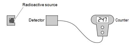
She put the radioactive source near the detector. She measured the number of counts in 20 seconds. She reset the counter to zero and measured the number of counts in the next 20 seconds. She continued this for 10 minutes.
