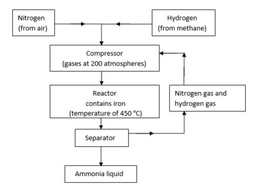
In the reactor the equation to produce ammonia is:
