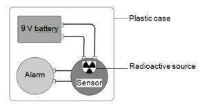
The alpha particles ionise the air inside the sensor, which causes a small electric current. Any smoke getting into the sensor will absorb alpha particles. This reduces the current. The change in current sets off the alarm.
