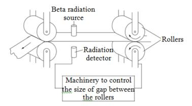
The paper passes through a narrow gap between a beta  $(\beta)$  radiation source and a detector.
