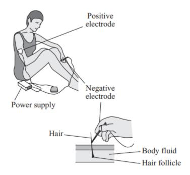
The hair is first coated with a layer of gel containing ions in solution. The positive electrode is connected by a patch to the skin. The negative electrode is connected to the hair. Electricity flows through the gel and causes electrolysis of the body fluid around the hair follicle.
