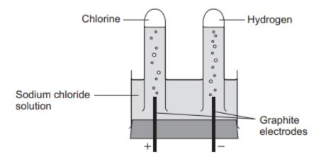
One of the products of the electrolysis of sodium chloride solution is hydrogen.
