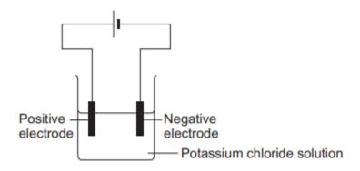
The student expected to see potassium metal at the negative electrode, but instead saw bubbles of a gas.
