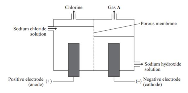
The electrolysis produces two gases, chlorine and Gas A. Name Gas A.
