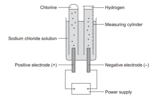
(a) Chlorine is produced at the positive electrode. Why are chloride ions attracted to the positive electrode?
