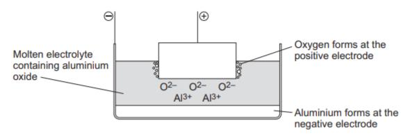
(a) The electrolyte is aluminium oxide mixed with another substance.
