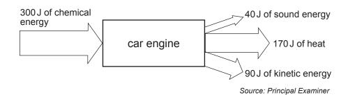
Calculate the efficiency of the engine.
