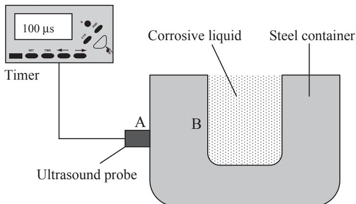
The ultrasound probe is placed in contact with the outside of the steel container at the point A. It then emits a pulse of ultrasound and 100 microseconds later detects the reflection of this ultrasound from the inner wall of the container at B.
