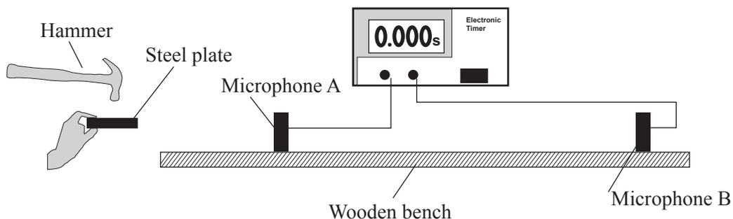
Describe how Roy could use the above apparatus to show that sound travels faster in wood than in air. State clearly what measurement would show that this is true.
