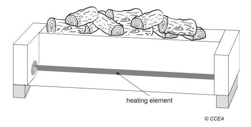
The heater has an electric power rating of 720 W when operated from a 240 V mains supply.
