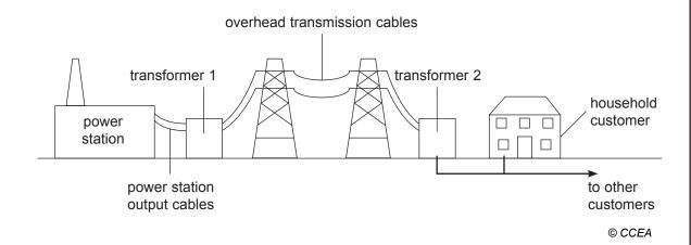
A power station generates electricity at a voltage of 15 kV. This is increased to 120 kV by transformer 1.
