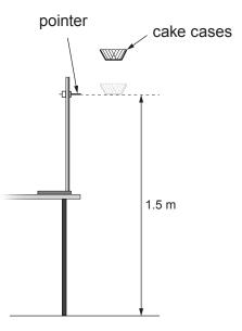
The cake cases are dropped from at least 20 cm above the pointer. This allows them to reach a terminal speed by the time they reach the pointer. The time taken for the cases to fall the distance of 1.5 m between the pointer and the floor is measured.
